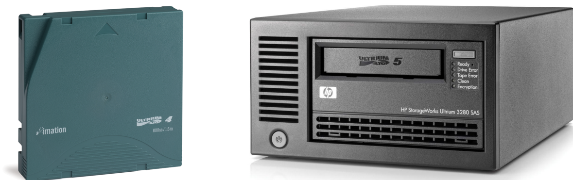
Figure 1: a LTO-4 tape and a LTO-5 reader/writer.
