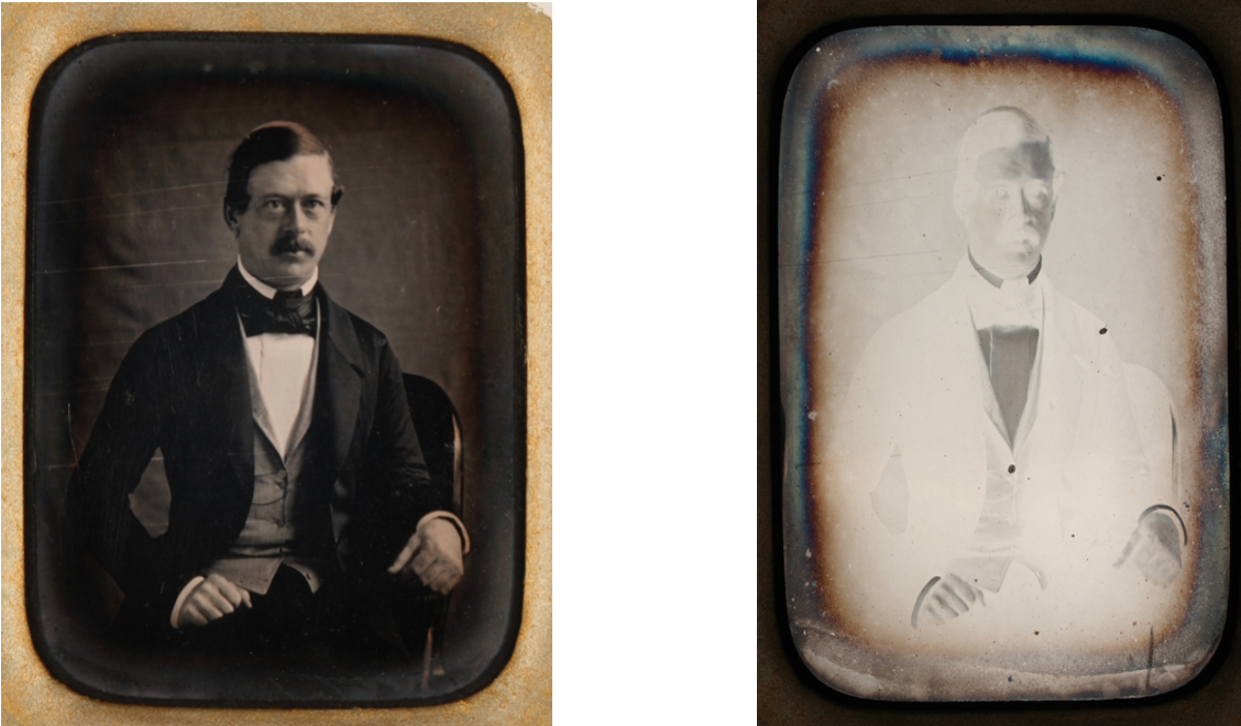
Image 6.1 and 5.2. Standard frontal illumination ( 45^\circ from left and right) and specular illumination (using a sheet of glass at 45^\circ between the camera and the object).
