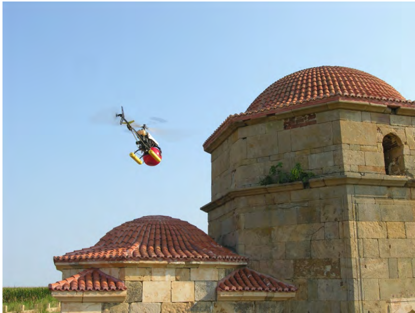
Fig. 13: the drone used by CETI to digitise buildings
